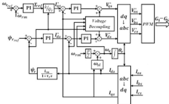
Fig.2. Block diagram of current controller for Grid connected mode
