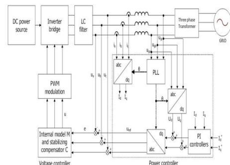
Fig.1. schematic diagram of grid-connected system
