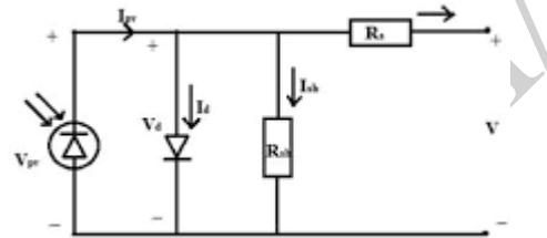
Fig 4: Single diode model of PV cell
