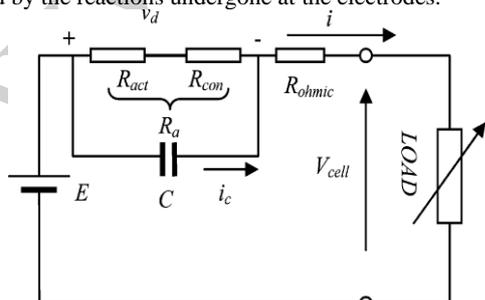
Fig 5: Equivalent circuit of PEMFC
