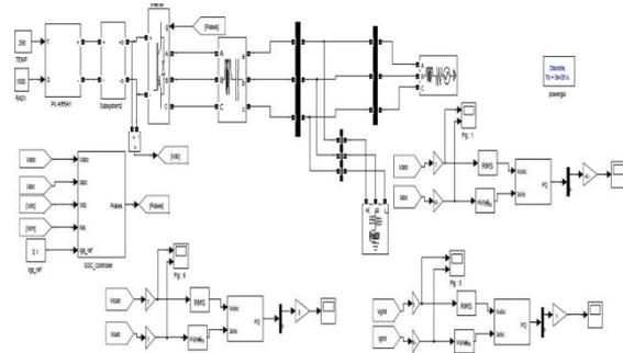
Fig 8. Islanding operation of Distributed generation
