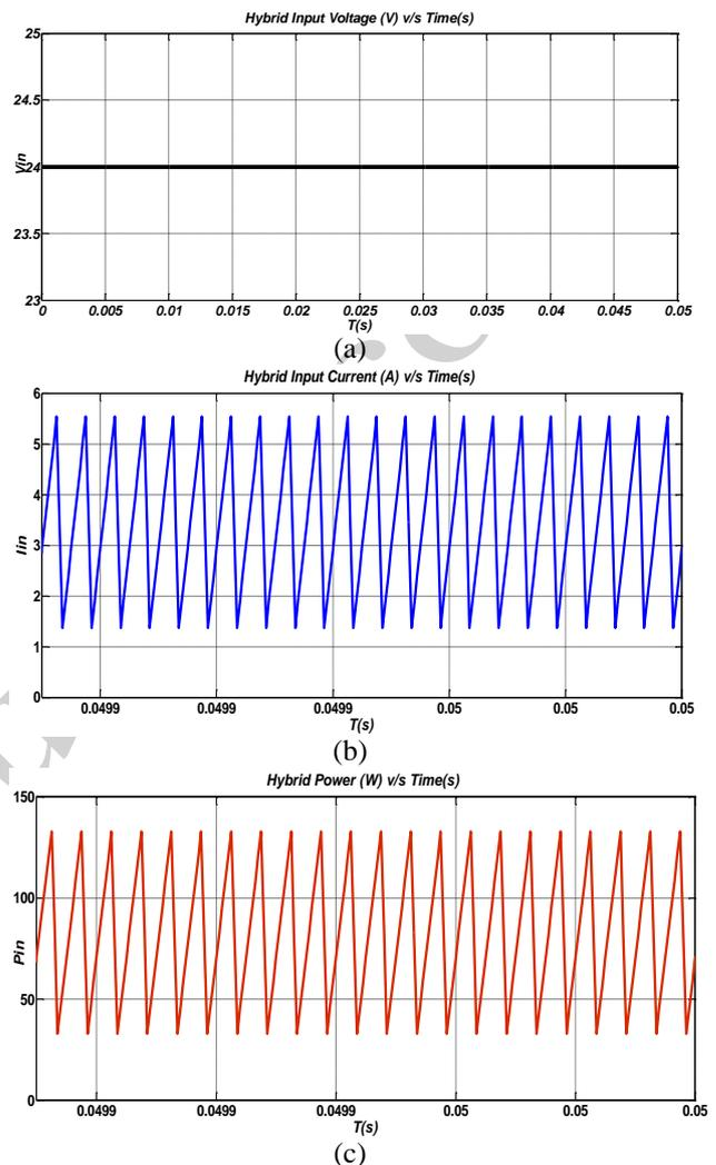
Fig.3. Simulated input Results for R-Load ( $R=21.62 \Omega$ ), R-L load( $R=21.62 \Omega, L=100\text{mH}$ ) and (a) $V_{in}$  (b)  $I_{in}$  (c)  $P_{in}$
