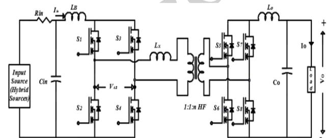
Fig.1 SST based isolated FBC for Hybrid E-V's
