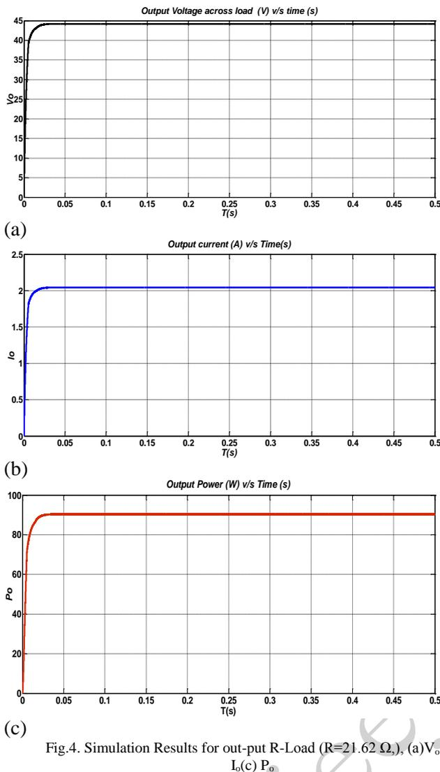
Fig.4. Simulation Results for out-put R-Load ( $R=21.62 \Omega$ ), (a)  $V_o$  (b)  $I_o$  (c)  $P_o$
