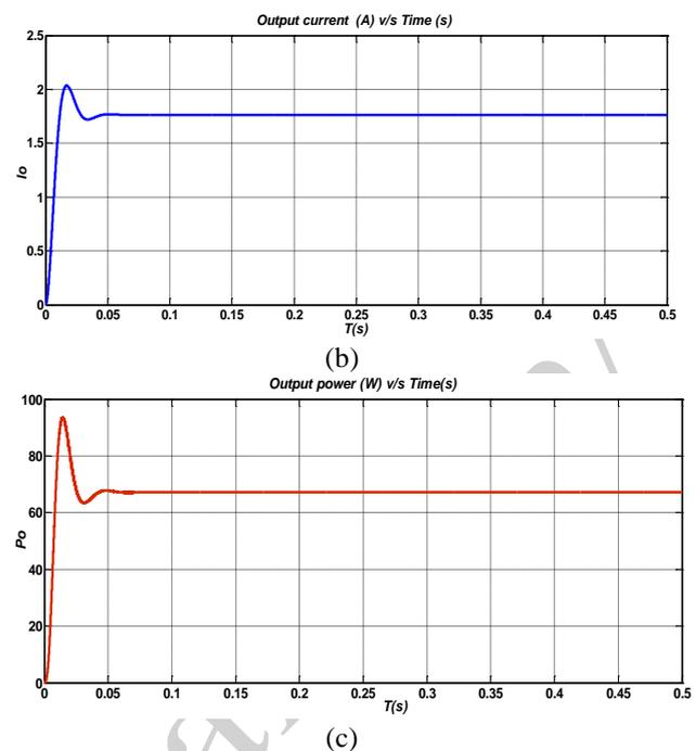
Fig.5 Simulation Results for out-put R-L load ( $R=21.62 \Omega, L=100mH$ ) (a)  $V_o$  (b)  $I_o$  (c)  $P_o$
