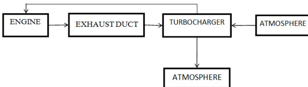
Fig. 2: Block diagram of Conventional Exhaust system of a diesel locomotive
