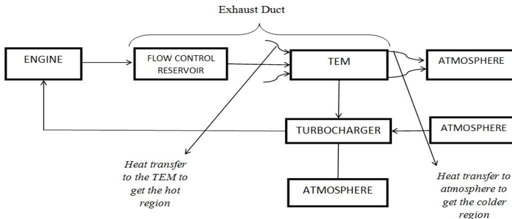
Fig. 3: Block diagram of Modified TEM Exhaust system of the Diesel Locomotive
