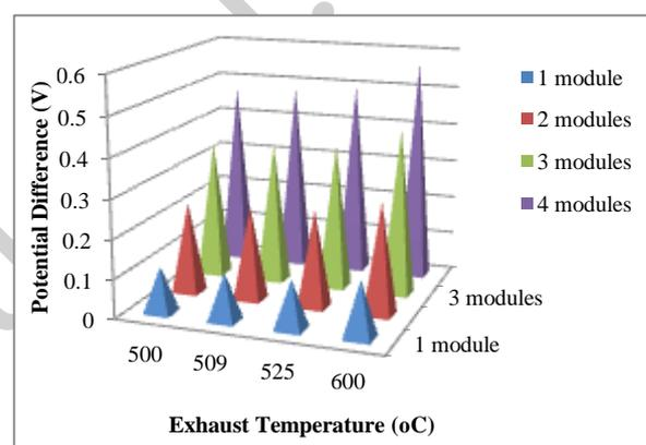
Fig. 6: Potential Difference Generated No. of Modules
